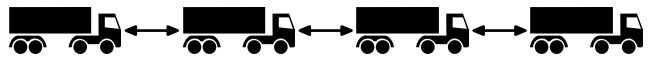
Fig. 4: A four agent vehicular platoon. The arrows indicate communication links between the agents.
