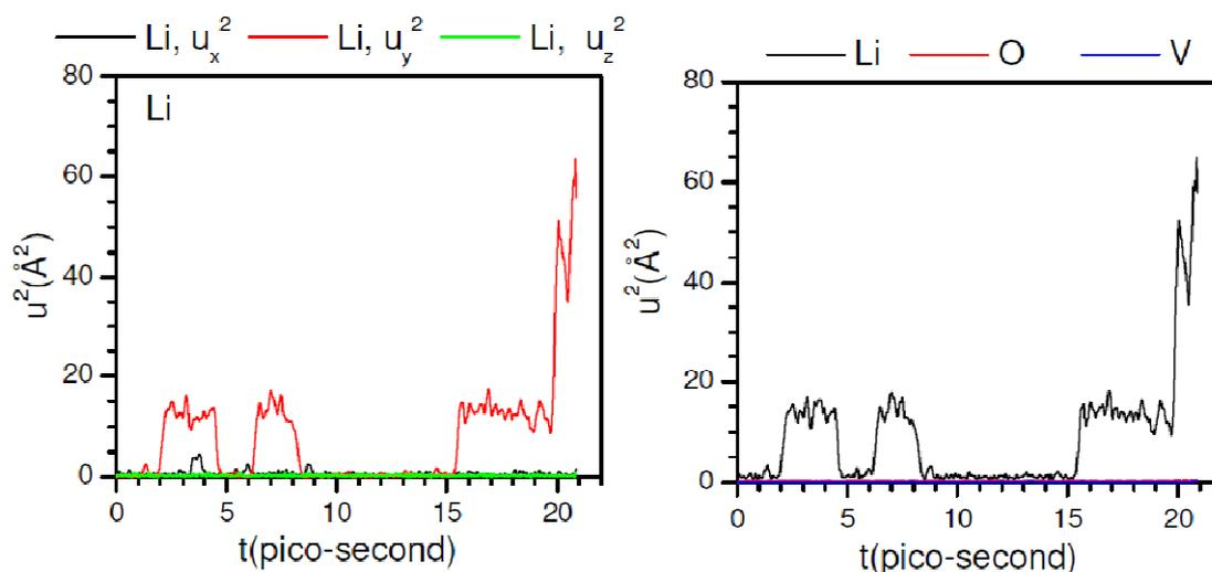
**FIG 4** (Left) The calculated squared displacement of Li atoms (Li1 & Li2) along the crystallographic axes at 1200K. (Right) The calculated mean squared displacement of various atoms Li1, Li2, O, Al in  $\text{Li}_{0.16}\text{V}_2\text{O}_5$  obtained from ab-initio MD simulations at 1200 K.
