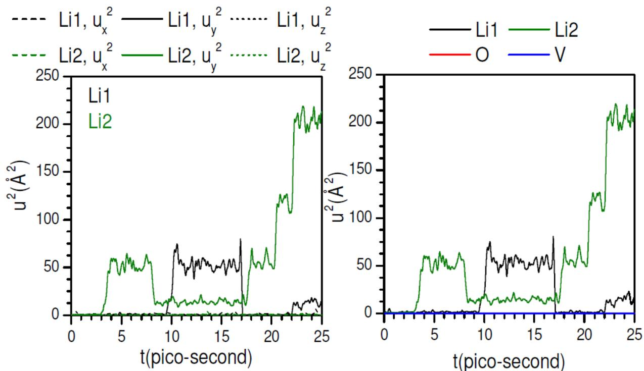
**FIG 5** The calculated trajectories of Li in (Left)  $\text{Li}_{0.08}\text{V}_2\text{O}_5$  and (Right)  $\text{Li}_{0.16}\text{V}_2\text{O}_5$  obtained from ab-initio MD simulations at 1200 K. The time dependent positions of Li atoms are shown by green and black dots. Key: O- Red & V-Blue.
