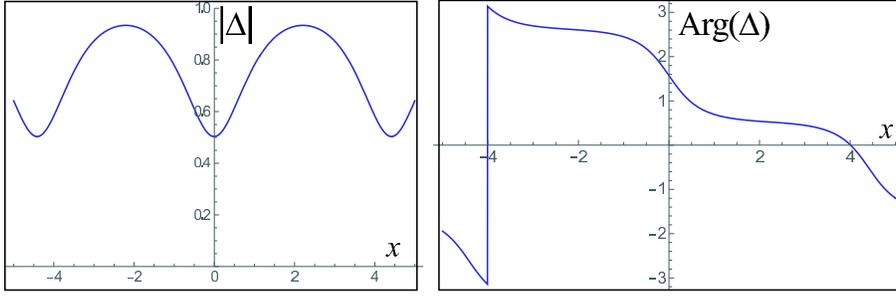
FIG. 6: The general solution of the NLSE. Both the amplitude and the phase modulate in space. The amplitude of the condensate does not touch to zero in the presence of the current. The modulation of the phase is also not uniform in the space.
