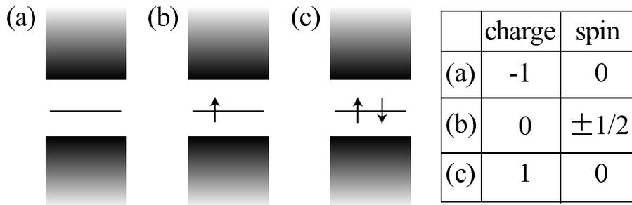
FIG. 5: The occupation number of the zero mode and the charge-spin separation. Fig. (a), (b), and (c), respectively, show the empty state, the singly occupied state, and the doubly occupied state. Those situations yield the charge-spin separation of the conducting degrees of freedom.
