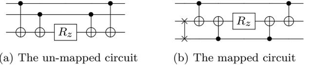
**Fig. 3.** An example of circuit transformation made by lookahead swap, one of **routing** passes. The first gate in circuit (b) is a quantum swap gate, which swaps the quantum state of the two connected qubits. Consequently, all the following gates operating on these two qubits have to swap the two operands.
