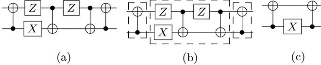
**Fig. 9.** A working example of `commutation_analysis` and `commutative_cancellation`. (a) The un-optimized circuit, (b) `commutation_analysis` forming the commutation groups, and (c) `commutative_cancellation` cancels self-inverse gates inside groups.
