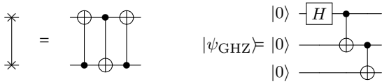
Fig. 1. Examples of circuit decomposition: SWAP gate decomposition (left); A circuit for preparing the 3 qubit GHZ state: |\psi_{\text{GHZ}}\rangle = \frac{1}{\sqrt{2}}(|000\rangle + |111\rangle) . (right).
