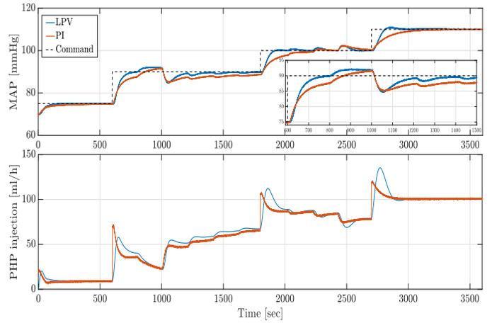
**FIGURE 5.** Closed-loop MAP response and control effort of proposed LPV controller against fixed structure PI controller subject to disturbance and measurement noise
