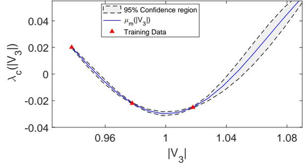
Fig. 1. An illustration on *GP-UCB* working on 1-D state subspace of  $|V_3|$ . The blue line denotes mean values of the unknown function  $\lambda_c(|V_3|)$ , and the gray shade describes the 95% confidence interval. The three red triangles represent three different sampling points.
