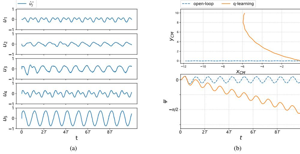
Fig. 8. Summary of control results: (a) The learned control input (26) from the Q-learning algorithm; (b) Time trace of the global displacement  $r_{CM} = (x_{CM}, y_{CM})$  and the global orientation  $\psi$  in open-loop manner ( $u(t) = 0$ ), and using the learned control input.
