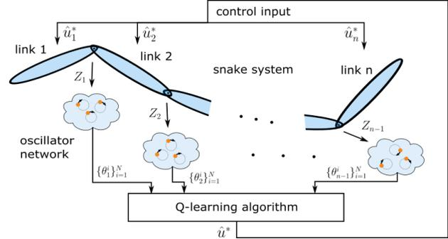
Fig. 1. The proposed architecture to learn a distributed feedback control law for turning the snake robot.
