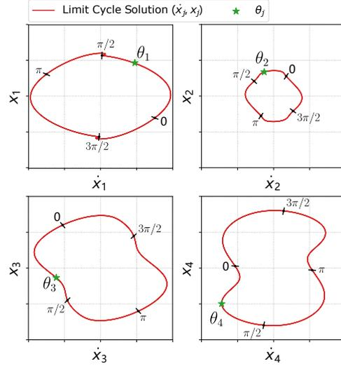
Fig. 3. The limit cycle solution for the shape variable  $(x(t), \dot{x}(t))$  under the periodic torque input (2), for a 5-link system. Each limit cycle is parameterized with a phase variable  $\theta_j \in [0, 2\pi]$ .
