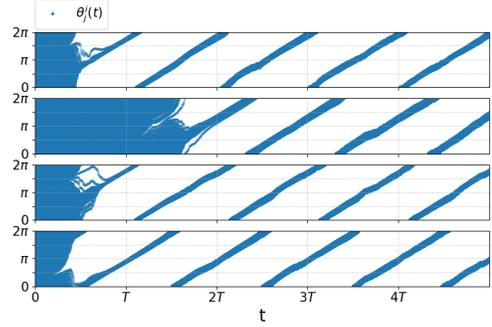
Fig. 6. Time trace of  $N = 100$  particles for the four independent FPF algorithm (24). The empirical distribution of the particles for the  $j$ -th FPF approximates the posterior distribution of the phase variable corresponds to the  $j$ -th joint of the 5-link system.
