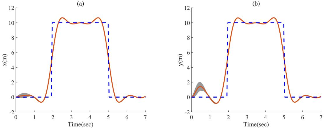
Fig. 4: The Quadrotor tracks step reference. (a): in  $x$  direction; (b): in  $y$  direction. Red line shows the mean controlled trajectory, the grey line show the effects caused by the uncertainties, and blue dotted line is the reference trajectory.
