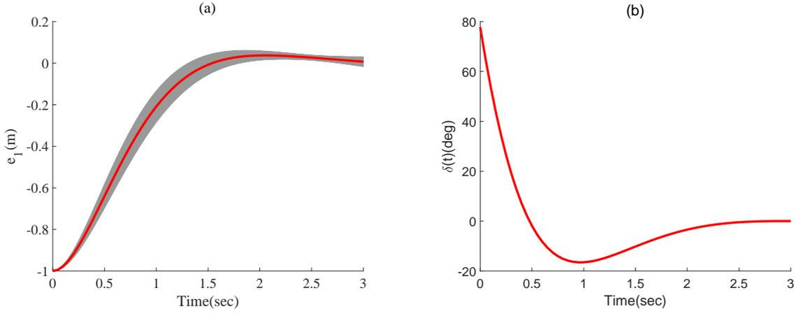
Fig. 3: Numerical results for vehicle path following experiment. (a): resulting lateral position error, where the red line shows the mean value, and the grey lines show the trajectory uncertainties; (b): Optimal control input  $\delta(t)$ .
