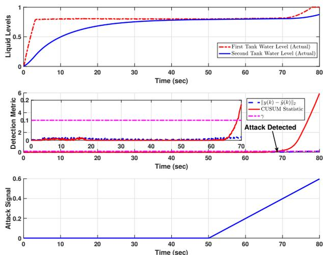
Fig. 5. Scenario in which the control input signal is compromised. In particular, the actual control signal  $u(k)$  is replaced with  $u(k) + u^a(k)$  where  $u^a(k)$  is the attack signal showed in the bottom graph. The attack signal is started at  $t = 50$  sec and detected at  $t = 6.9$  sec.
