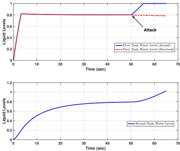
Fig. 2. Scenario in which the reading from the level sensor reporting liquid level in Tank 1 is compromised starting from time  $t = 50$  sec. The top figure shows both the actual, as well as the deceived liquid levels in Tank 1. The bottom figure presents the liquid level at Tank 2. A simple false data injection attack causes both tanks to overflow.
