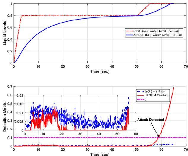
Fig. 4. Same scenario as the one in Fig. 3, but in the presence of added white Gaussian noise. The performance of the controller/detector is not affected by noise.
