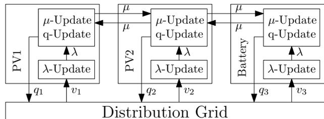
Fig. 3: Control architecture. Measurement and actuation is performed locally by each controller. Only the dual multipliers  $\mu_{\min}$  and  $\mu_{\max}$  need to be communicated to neighboring peers.
