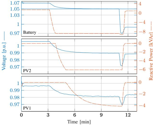
Fig. 7: Performance of the distributed voltage controller,  $\alpha = 100$ .
