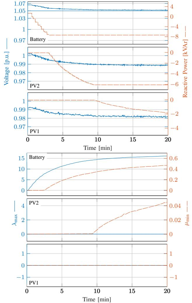
Fig. 8: Behavior of the distributed controller with control gain  $\alpha = 50$ . Upper panels: electrical quantities  $v, q$ . Lower panel: dual multipliers  $\lambda_{\max}$  and  $\mu_{\min}$  (evaluated at the last step of Algorithm 2).
