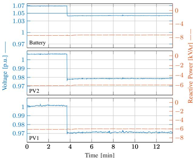
Fig. 10: Controller windup due to a persistent overvoltage.
