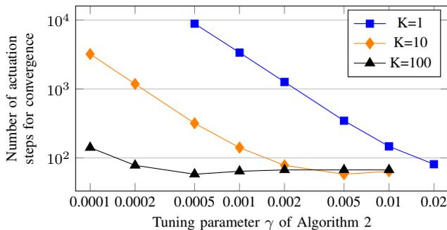
Fig. 12: Number of actuation steps required for convergence as a function of  $\gamma$  and of the number of communication steps  $K$ . Network with 3 inverters and  $\alpha = 100$ . Each curve stops, at the right end, at the largest  $\gamma$  that does not cause instability.
