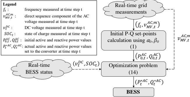
Fig. 4. Block diagram of the proposed real-time controller.
