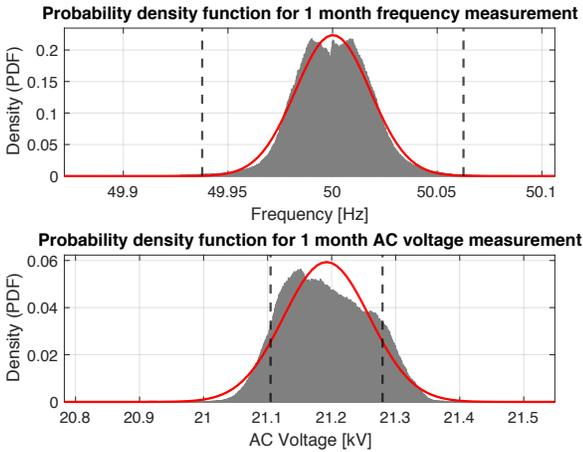
Fig. 6. 1 month historical data of frequency and phase-to-phase voltage at the BESS PCC at 21 kV, acquired via PMUs installed at the EPFL MV network. The dashed lines represent the limits of  $\mu_f \pm 3.3\sigma_f$  and  $\mu_V \pm 1\sigma_V$  for frequency and voltage measurements, respectively.
