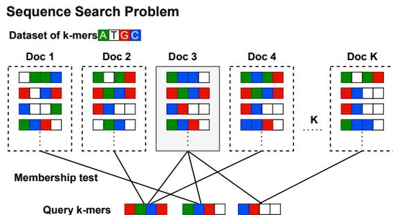
**Figure 1: Sequence search problem: First, we convert each of the  $K$  documents into a set of  $k$ -mers. The  $k$ -mers of length 31 are generated using a sliding window on the sequence ( $k=4$  in the figure for illustration). Given the  $k$ -mers from a query sequence, the task is to determine which of the  $K$  documents contain all the  $k$ -mers present in the query.**
