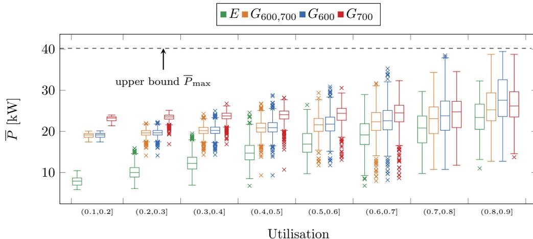
**Figure 9.** Average power per idle time  $\bar{P}$  depending on the modelling of the machine dynamics and utilisation of the machine.
