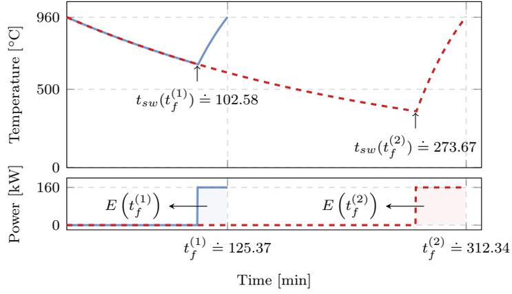
**Figure 6.** Example of the optimal control for two different terminal times  $t_f^{(1)}$  and  $t_f^{(2)}$ .
