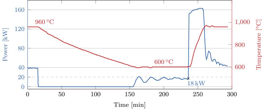
**Figure 4.** Relationship between the temperature and power when cooling to 600 °C and heating back to operating temperature
