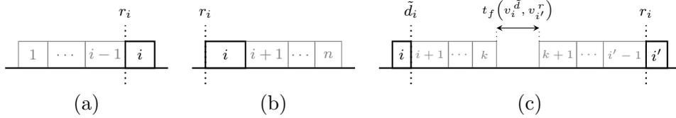
**Figure 1.** Examples of the partial schedules corresponding to the edges between (a)  $(v^s, v_i^r)$ , (b)  $(v_i^r, v^e)$ , and (c)  $(v_i^{\bar{d}}, v_{i'}^r)$ .
