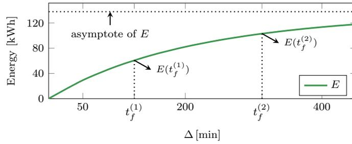
**Figure 7.** Idle energy function  $E$  and two different idle period lengths  $t_f^{(1)}$  and  $t_f^{(2)}$  with the corresponding idle energy consumption  $E(t_f^{(1)})$  and  $E(t_f^{(2)})$ .
