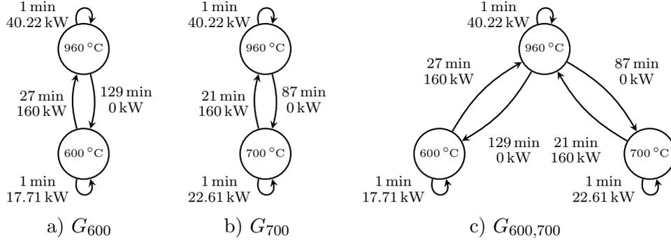
**Figure 8.** Examples of the transition graphs for the furnace model (14) with parameters (40).
