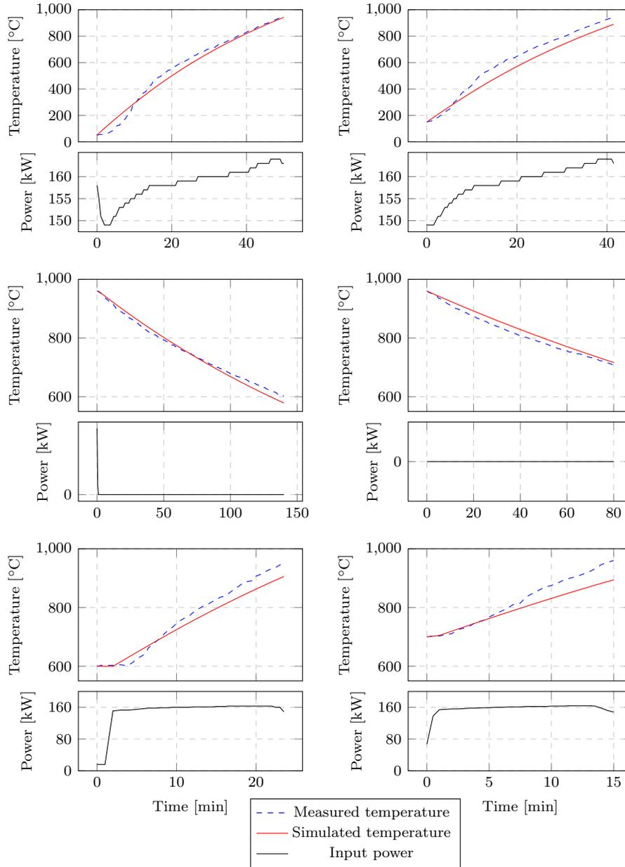
Figure 5. Comparison of the measured data and simulation using a bilinear model.
