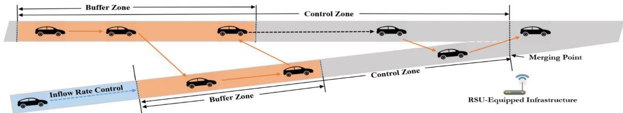
Fig. 1 Illustration of different zones of the proposed optimal control-based ramp merging system
