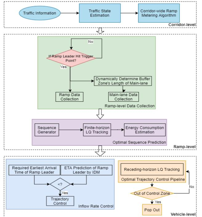
Fig. 2 Flow chart of the proposed ramp merging system
