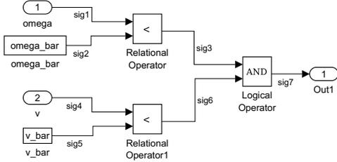
Figure 4: An implementation of the STL specification  $(\omega < \bar{\omega}) \wedge (v < \bar{v})$ , which is interpreted as “The engine speed  $\omega$  and the vehicle speed  $v$  never reach  $\bar{\omega}$  and  $\bar{v}$ , respectively”.
