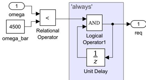
Figure 2: A simple example of a specification expressed in Simulink. The natural language interpretation is “During all simulation times  $t \in [0, T]$ , the engine speed  $\omega$  never reaches  $\bar{\omega}$ ”. For the implementation to be correct, the initial condition of the *Unit Delay* block must be non-zero.
