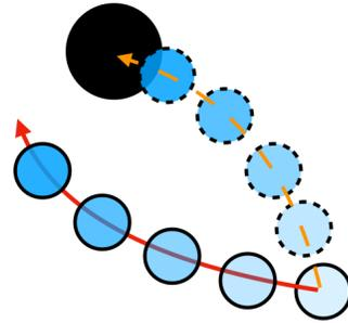
Fig. 1: An illustration of MPS. If using  $\hat{\pi}$  (dashed orange line), the robot (blue) may unsafely crash into the obstacle (black). Using  $\pi_{\text{backup}}$  (solid red line) ensures safety.
