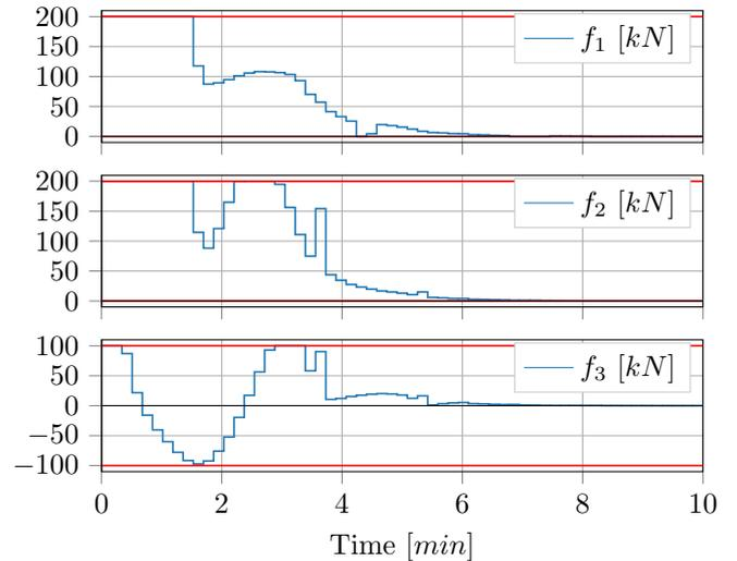
Fig. 10. Thruster force for docking at Trondheim harbour, with saturation constraints indicated in red.
