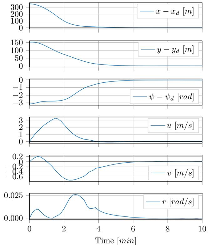
Fig. 6. Vessel pose error  $\eta - \eta_d$  and velocity  $\nu$  when docking at Lundevågen harbour.
