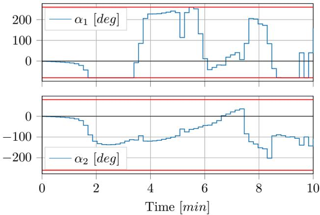
Fig. 8. Azimuth angles when docking at Lundevangen harbour, with saturation constraints indicated in red.
