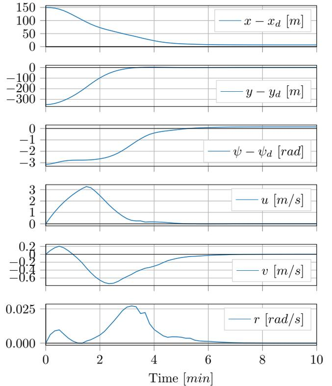
Fig. 9. Vessel pose error  $\boldsymbol{\eta} - \boldsymbol{\eta}_d$  and velocity  $\boldsymbol{v}$  when docking at Trondheim harbour.
