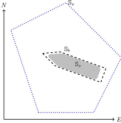
Fig. 3. Vessel  $\mathbb{S}_v$  with safety boundary  $\mathbb{S}_b$  with black dashed line, and spatial constraints  $\mathbb{S}_s$  as blue dotted line, in the NED frame. The vessel will always lie within the spatial constraints  $\mathbb{S}_s$  as long as all the vertices of  $\mathbb{S}_b$  lie within the spatial constraints.
