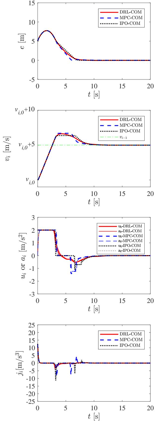
Fig. 4. Testing results when there are no modeling errors for the single initial condition considered. In the plots, MPC  $h=2.8\text{s}$ . When MPC  $h=5\text{s}$ , the MPC results are almost identical to those of IPO. The symbol  $v_{i,0}$  denotes the initial velocity of the following vehicle  $i$ .
