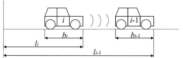
Fig. 2. Schematic for two-car following.
