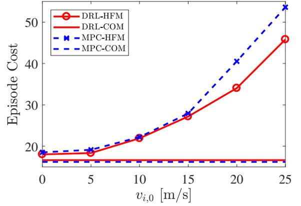
Fig. 9. Episode cost for constant-speed following for the single initial condition considered. In the plot, MPC  $h=5\text{s}$ .
