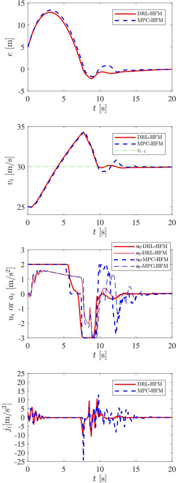
Fig. 8. HFM test results for constant-speed following for the single initial condition considered. The initial velocity of the following vehicle is  $v_{i,0}=25\text{m/s}$ . In the plots, MPC  $h=5\text{s}$ .
