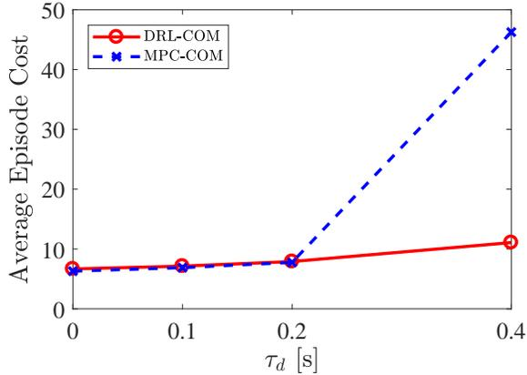
Fig. 7. Average episode cost for different control delay  $\tau_d$  values. The control delay was added to the COM for testing.
