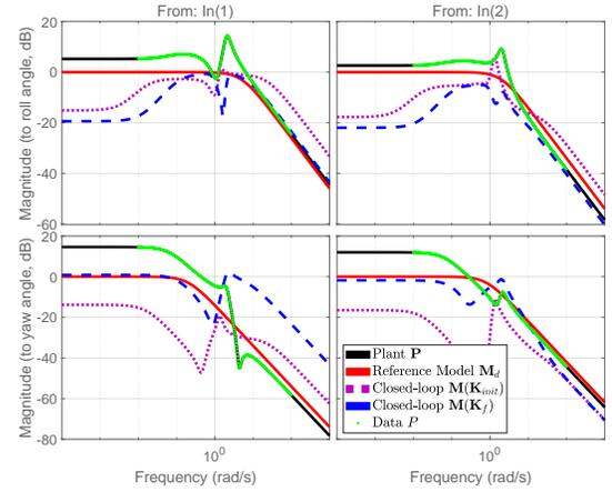
Fig. 4. Closed-loop transfers for the angle control f16 air fighter
