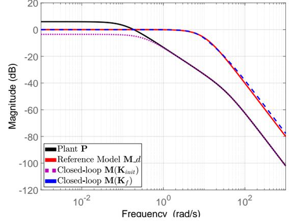
Fig. 3. Closed-loop transfers in the DC motor case.
