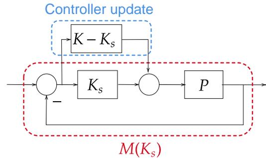
Fig. 2. Equivalent interconnection to the resulting closed-loop visible on Figure 1 based on a stabilizing controller  $\mathbf{K}_s$ , allowing to use the small-gain theorem.
