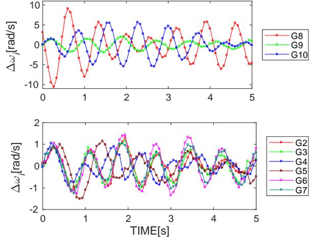
Fig. 2: Rotor speed deviations of generators 2–10 in the New England test grid. These are the trajectories of (27) for the initial condition (28) and contain additive i.i.d. noise.
