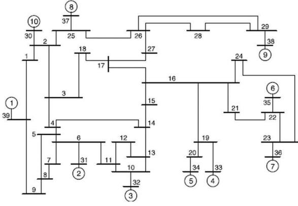
Fig. 1: New England 39-bus test grid (NE grid)
