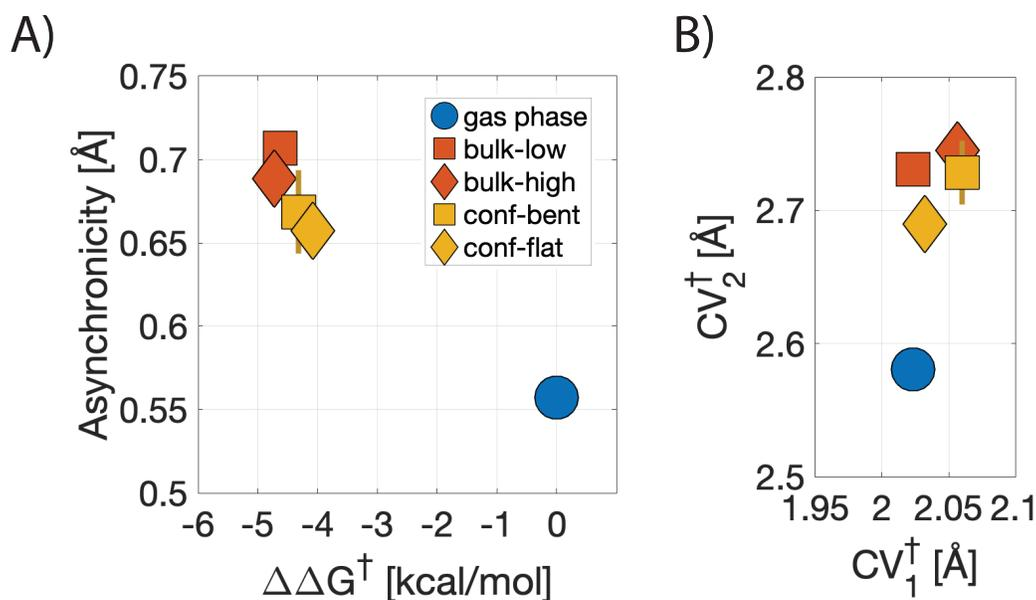
**Figure 2. Transition state asynchronicity for the CPD-MVK retro-DA reaction.** (a) Asynchronicity  $\Delta CV^\ddagger$  as a function of the activation free energy  $\Delta\Delta G^\ddagger$ . (b) Values of the collective variables when the system is at the transition state. All environmental reaction conditions show similar activation free energies and mechanism within error bars.
