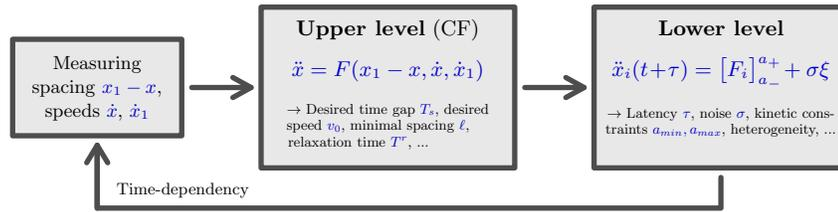
**Fig. 2.** Operational scheme for ACC systems. At upper level control, ACC systems are stable car-following models based on desired time gap, desired speed or relaxation time parameters. At lower level control, factors such as delay and latency, noise and measurement error, heterogeneity and kinetic constraints affect the dynamics and may even break the stability.
