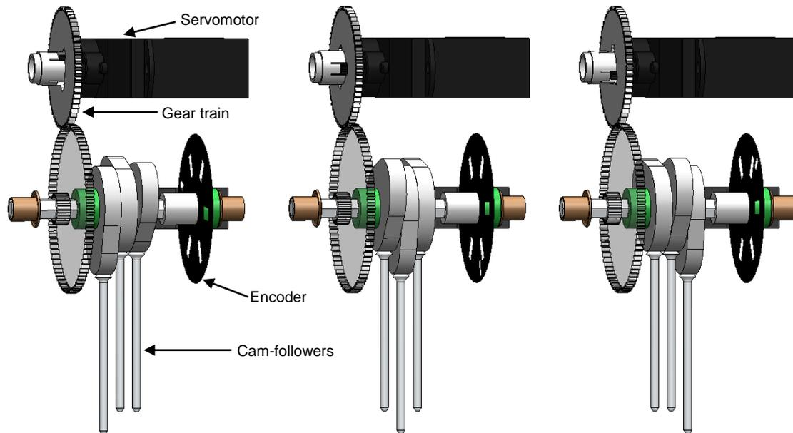
Figure 2: Detail of the embossing system. Three cam-follower mechanisms are arranged at 120° intervals around the shaft and their actuation is determined by the rotation of the servomotor.
