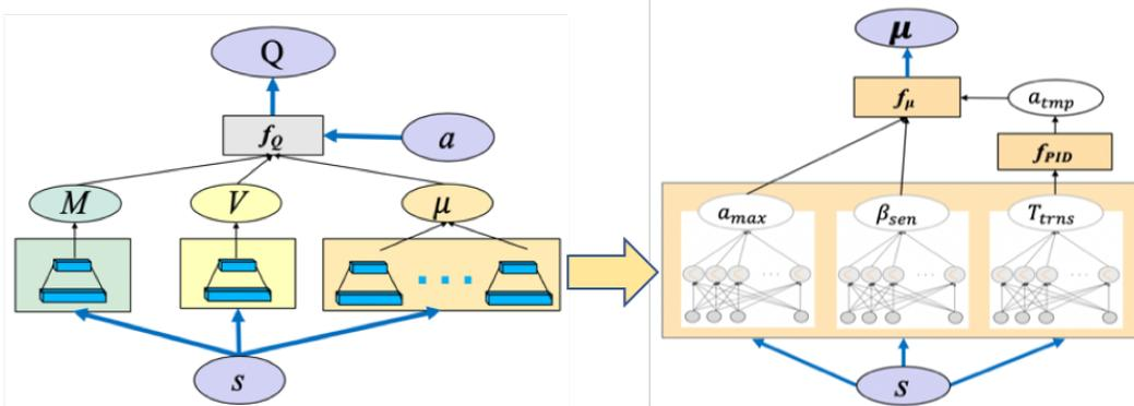
Figure 1: Architecture of Quadratic Q-network (left) and action network  $\mu$  (right).
