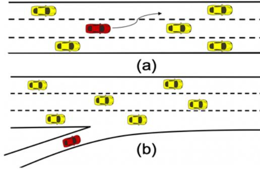
Figure 2: (a) Lane-change scenario (b) Highway ramp-merge scenario.
