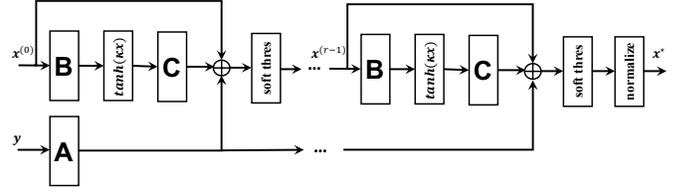
Fig. 1. The block diagram of the proposed DeepFPC.
