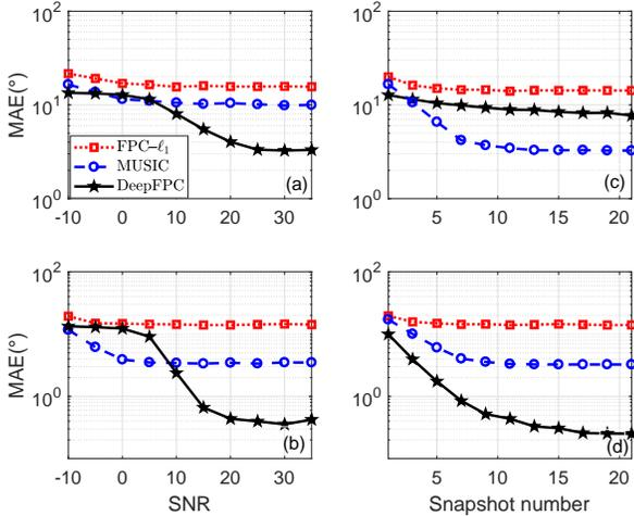
Fig. 3. DOA estimation error for three methods ( $M = 40$ ): (a) MAE versus SNR with snapshot number  $L = 3$ ; (b) MAE versus SNR with snapshot number  $L = 10$ ; (c) MAE versus snapshot number  $L$  with SNR=5dB and (d) MAE versus snapshot number  $L$  with SNR=20dB.
