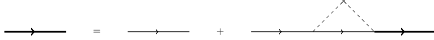
Figure 1: The leading order correction to the electron Green's function due to impurity averaging. The thin solid line is the free electron Green's function; the thick solid line is the impurity dressed electron Green function; the dashed line denotes correlated impurity scattering events.
