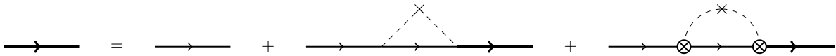
Figure 5: The diagrammatic series for the electron Green's function in a granular system. The additional term relative to fig. 1 is due to correlated tunnelling back and forth between neighbouring grains.
