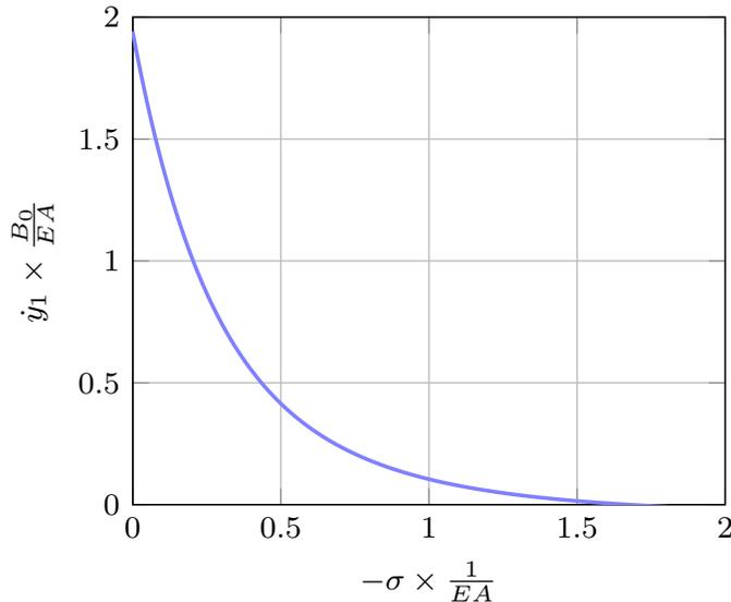
Figure 11: Example of evolution of the growth velocity of the bar approaching treadmilling.  $W^*(\sigma)$  from eq. (57) with parameters  $\sigma_{\text{asympt}} = 2EA$ ,  $\sigma_{\text{max}} = 0EA$ ,  $\sigma_{\alpha 0} = -4EA$ ,  $\sigma_{\alpha 1} = -1EA$ ,  $\beta = 1.0$ .
