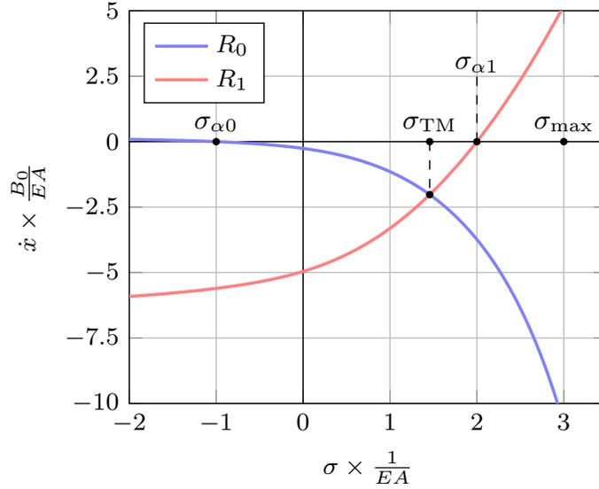
Figure 4: Example of treading solution obtained using  $W^*(\sigma)$  from eq. (57) with parameters  $\sigma_{\text{asympt}} = 5EA$ ,  $\sigma_{\text{max}} = 3EA$ ,  $\sigma_{\alpha 0} = -EA$ ,  $\sigma_{\alpha 1} = 2EA$ ,  $\beta = 1.0$ .
