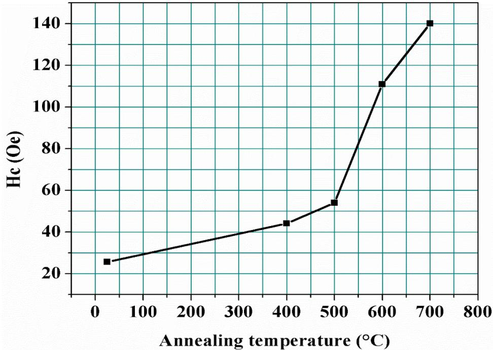
Fig.#6: Graph between annealing temperature and coercivity  $H_c$
