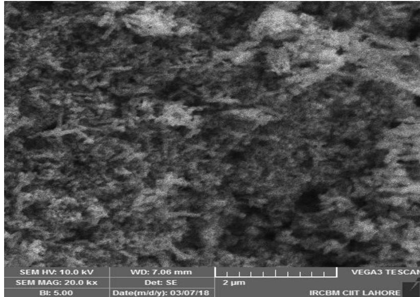
The SEM images show that the as deposited particles are more agglomerated but when the samples have been annealed at 700°C the agglomeration reduces because of heat treatment. As prepared samples looked having flake like shapes while the samples annealed at 700°C showed a rod like shape morphology. So, this implies that because of heat treatment there happened a longitudinal growth of the particles resulting in rod like structures at 700°C.
