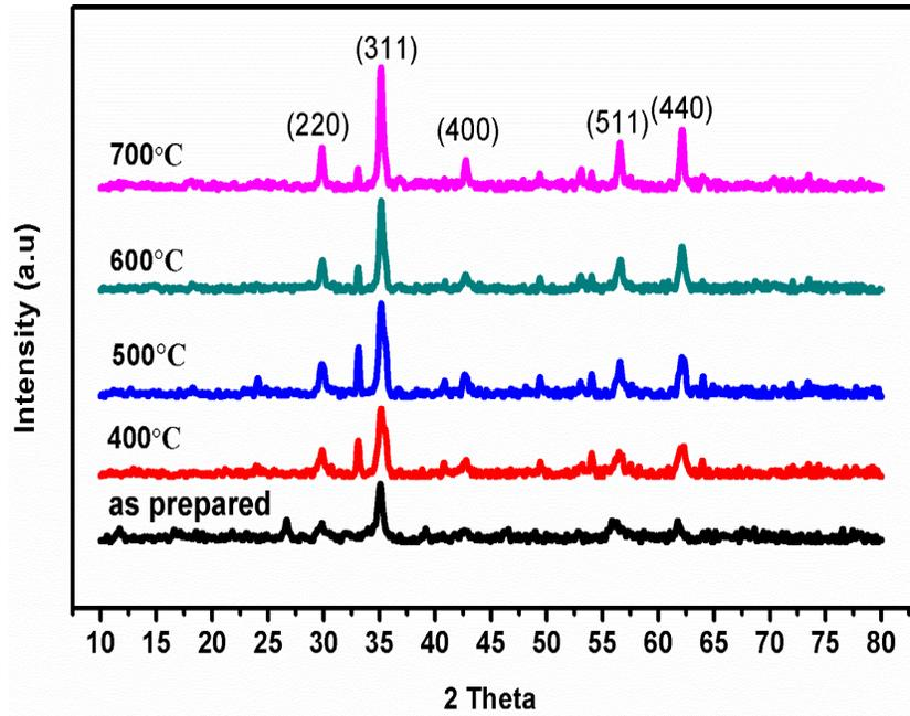
Fig#1 Indexed XRD patterns at different temperatures
