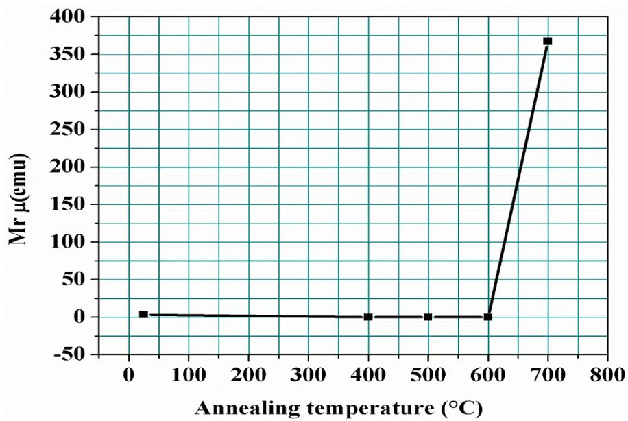
Fig.#5 Graph between annealing temperature ( $^{\circ}\text{C}$ ) and Retentivity ( $M_r$ )  $\mu\text{emu}$
