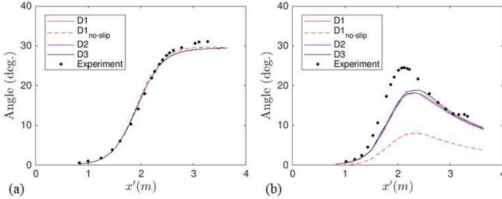
FIGURE 3. Crossflow turning angles: (a) freestream turning angle ( $\gamma_\infty$ ) distribution along the streamwise direction ( $x'$ ); (b) surface crossflow angle relative to freestream ( $\gamma_s - \gamma_\infty$ ) along the streamwise direction ( $x'$ ). Lines, present WMLES (cases D1, D2, D3); circles, experiment (Schwarz & Bradshaw 1994); dashed lines, no-slip LES on the case D1 mesh (without wall model).
