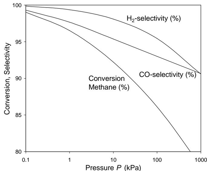
*Figure 2.* Thermodynamic equilibrium in adiabatic operation of air-based CPO of methane (no steam,  $O_2/C=0.5$ , air: 21 mol%  $O_2$ , 79%  $N_2$ ),  $T_{inlet}=300$  °C. Methane conversion and selectivities to CO and H<sub>2</sub> as function of pressure.
