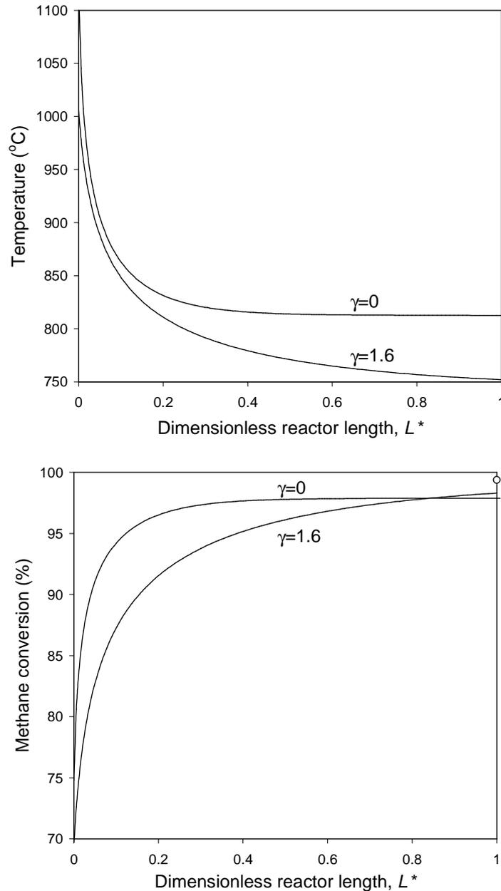
*Figure 6.* Temperature profile (a) and methane conversion (b) as function of reactor coordinate,  $L^*$ , for two steam-to-carbon ratio's,  $\gamma$ . The circle shows the equilibrium value for  $\gamma=1.6$  ( $\alpha=0.57$ ,  $P=150$  kPa,  $\phi_{\text{CH}_4,0}=10$  mmol/s,  $T_0=400$  °C,  $\lambda=0.10$  mol/(Pa·s),  $E_A=100$  kJ/mol,  $Q_{\text{ox}}=0$  W,  $\kappa=0$  W/K).
