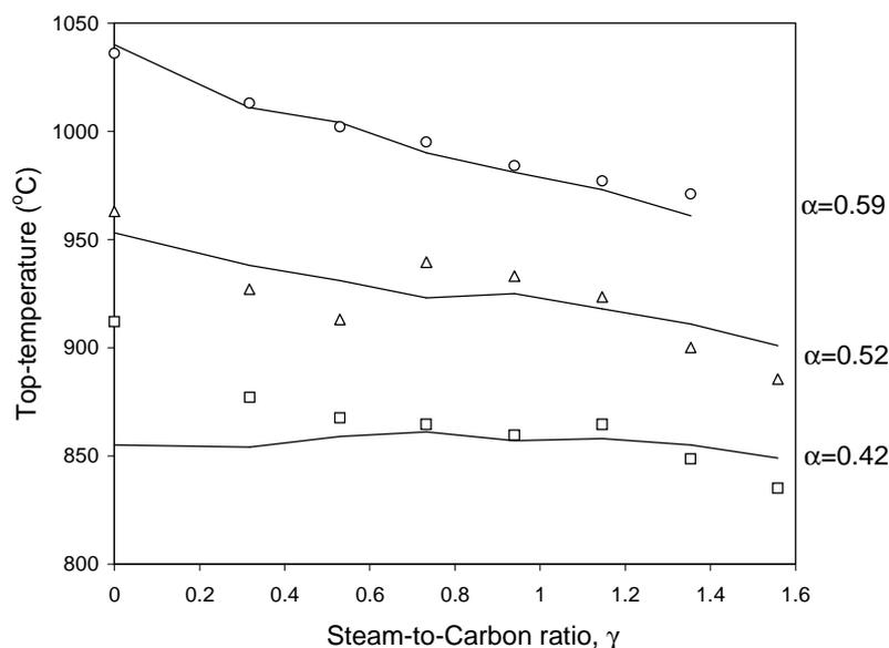
*Figure 3.* Top-temperature in ATR/CPO of methane. Different steam-to-carbon ratio's,  $\gamma$ , and oxygen-to-carbon ratio's,  $\alpha$ .  $T_0 \sim 400$  °C,  $P=150$  kPa, varying heat loss. Lines are predictions of the oxidation model.
