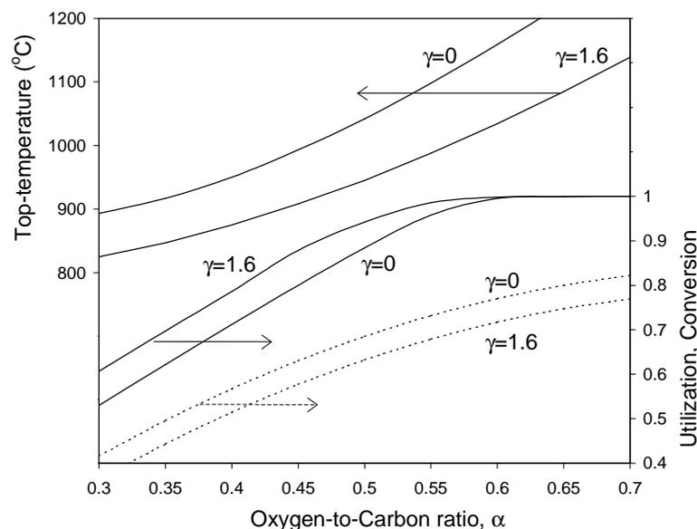
*Figure 5*. Oxidation Section in ATR/CPO of methane. Variation of oxygen-to-carbon ratio,  $\alpha$ , and steam-to-carbon ratio,  $\gamma$ . Top-temperature on left y-axis. Thermodynamic conversion (solid lines on right y-axis) as well as the fuel utilization (dashed lines).  $T_0 = 400$  °C,  $Q_{ox} = 0$  W,  $P = 150$  kPa.
