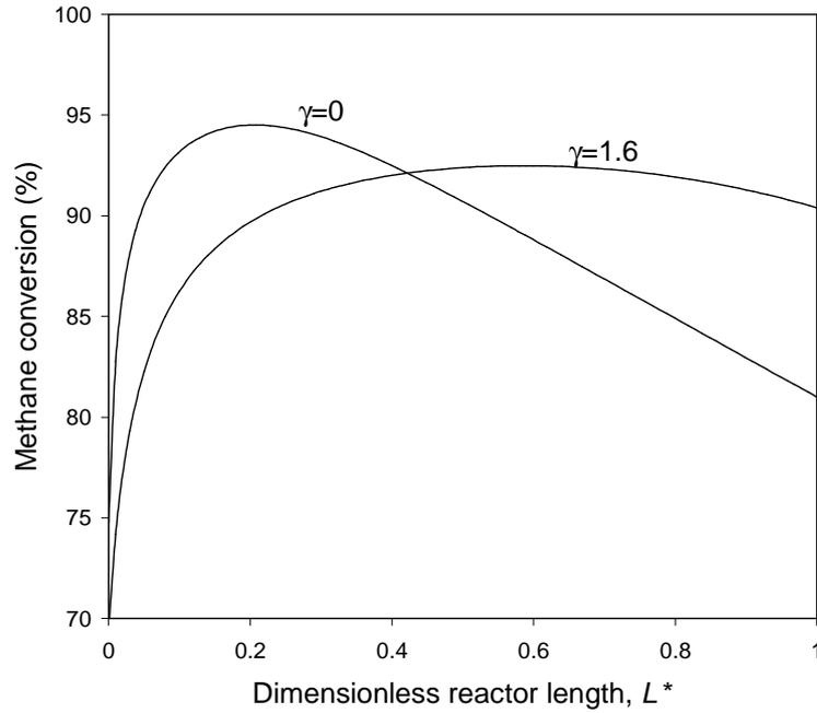
Figure 7. Methane conversion with heat loss in the reforming section, as function of  $\gamma$  and  $L^*$ . ( $\kappa=1$  W/K,  $T^*=298.15$  K, all other data see Figure 6).
