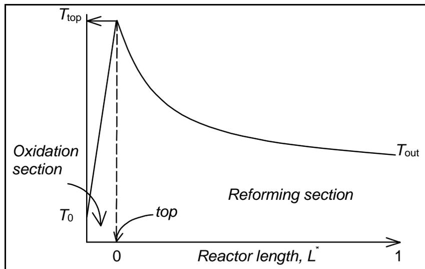
Figure 1. Gas phase temperature in CPO/ATR of methane. The measured *catalyst* temperature at the upstream side is assumed equal to the *gasphase* temperature at the intersection of the oxidation and reforming section (0, “top”).
