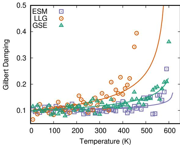
FIG. 9. (Color online) Temperature dependence of the Gilbert damping extracted from fitting the FMR line-shape. At low temperature the Gilbert damping is close to the atomistic damping value ( $\lambda = 0.1$ ), while it diverges as we approach the Curie temperature.
