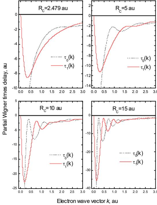
Fig. 1. Wigner times delay for  $C_2$  molecule versus electron wave vector  $k$  calculated within the model of non-overlapping atomic spheres.  $R_c$  is the inter-atomic distance.
