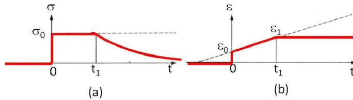
Figure 11: Stress and strain variation with time in the Standard Test for Maxwell Model
