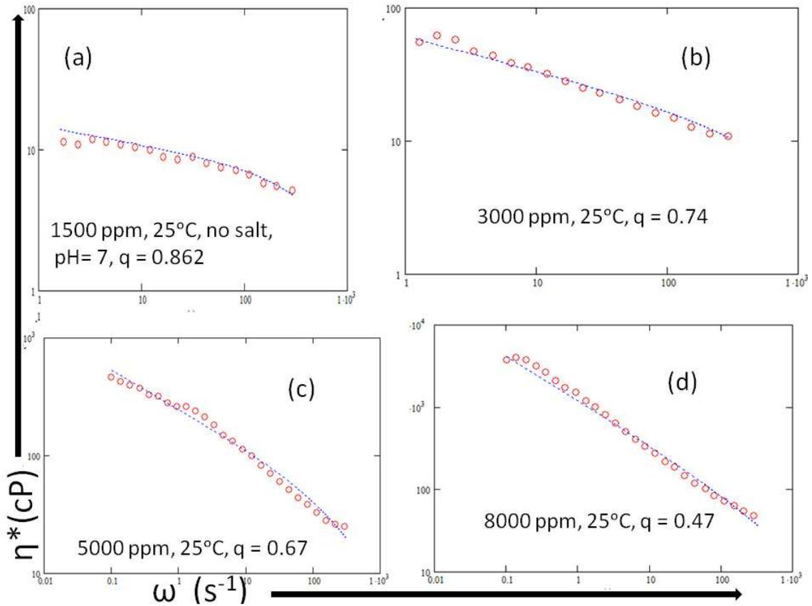
Figure 7: Variation of complex viscosity versus angular frequency for different polymer concentrations at constant temperature of 25°C, pH=7 and zero salinity, (a)1500 ppm (b)3000 ppm (c) 5000 ppm (d) 8000 ppm. Comparison between experiment and theory is good in each case.<sup>32</sup> The order of the fractional derivative decreases with increase in concentration as displayed in the graph.
