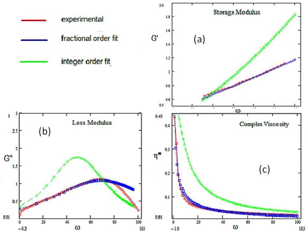
Figure 2: The rheological properties of HPAM obtained from experimental data compared with calculated values using Maxwell's Model using integer derivative and fractional derivative calculus.<sup>30</sup> (a) Storage modulus (b) Loss modulus (c) Complex viscosity. In all cases, the fractional derivative calculus fitted best the experimental data.
