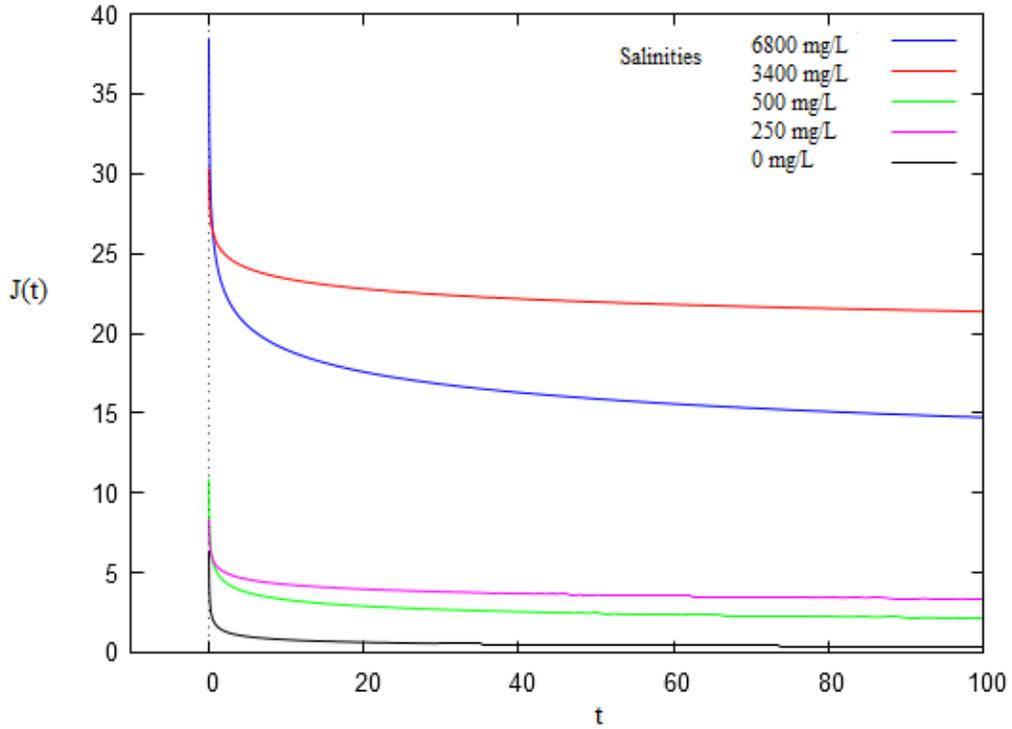
Figure 5: Variation of creep compliance with time for different salinities as predicted from theory
