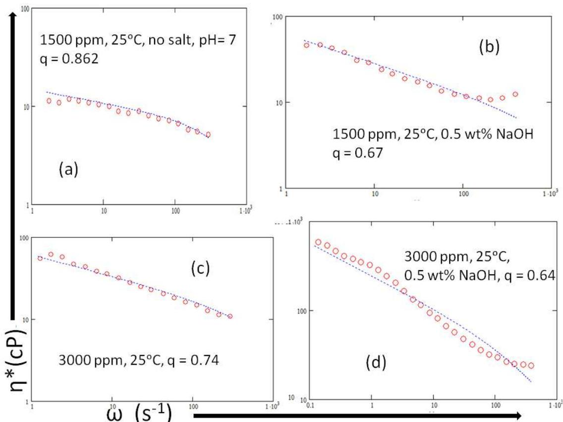
Figure 8: Variation of complex viscosity versus angular frequency for different pH. Experimental data from have been modelled.<sup>32</sup> (a) and (b) show the effect of pH for a polymer concentration of 1500 ppm at constant temperature of 25°C and zero salinity. (c) and (d) show the effect of pH for a polymer concentration of 3000 ppm at constant temperature of 25°C and zero salinity. The order of the fractional derivative decreases with increase in the alkalinity.
