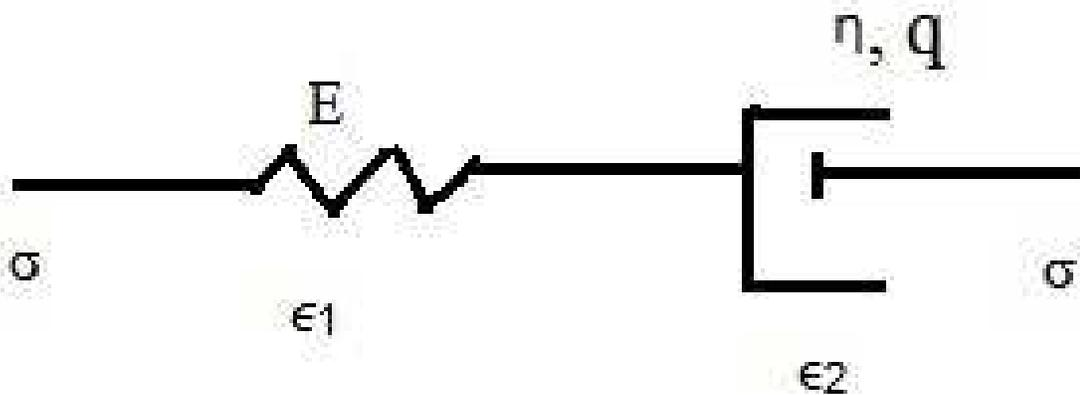
Figure 1: Schematic Maxwell model.  $E$  is the spring constant and  $\eta$  represents the viscosity of the fluid in the dashpot. For a stress  $\sigma$ ,  $\epsilon_1$  is the strain the the spring and  $\epsilon_2$ , that in the dashpot.
