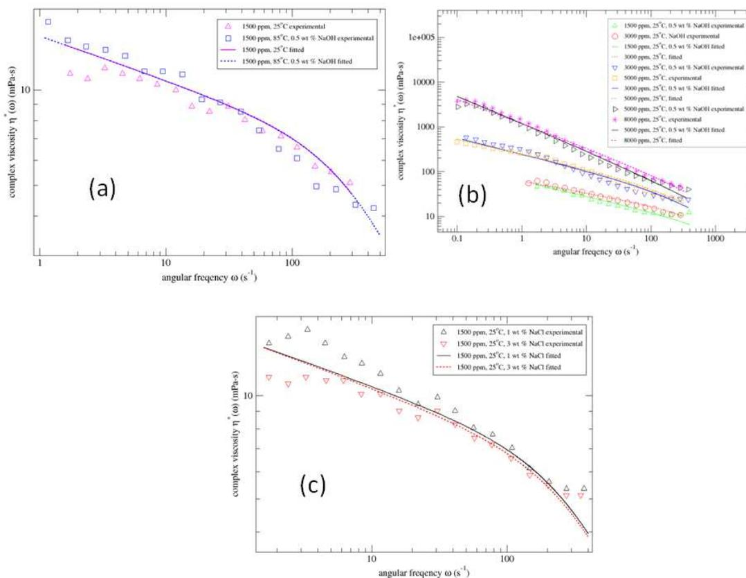
Figure 9: Variation of complex viscosity versus angular frequency for different combinations of *complementary conjugates*. Experimental data from Choi et al. have been modelled.<sup>32</sup> (a) Higher temperature is offset by a suitable increase in pH. (b) Effect of increased polymer concentration offset by lower the pH value. (c) Variations in salt concentration alone cannot offset small changes in concentration.
