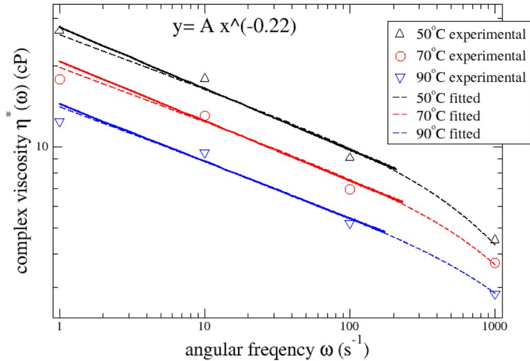
Figure 6: Variation of complex viscosity versus angular frequency for different temperatures: comparison between experiment and theory.<sup>31</sup> For angular frequencies  $\sim 120 \text{ s}^{-1}$ , the variation follows a power law with exponent of 0.22 for every temperature. The power law fit is shown by thick solid line.
