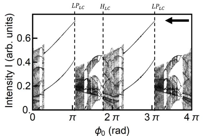
FIG. 5. Time-average extrema of  $I(t)$  obtained numerically for the negative direction of the frequency sweep for low amplitude bursting. The black arrow indicates the direction of sweep. The fixed parameters and the marks are the same as in Fig. 4.
