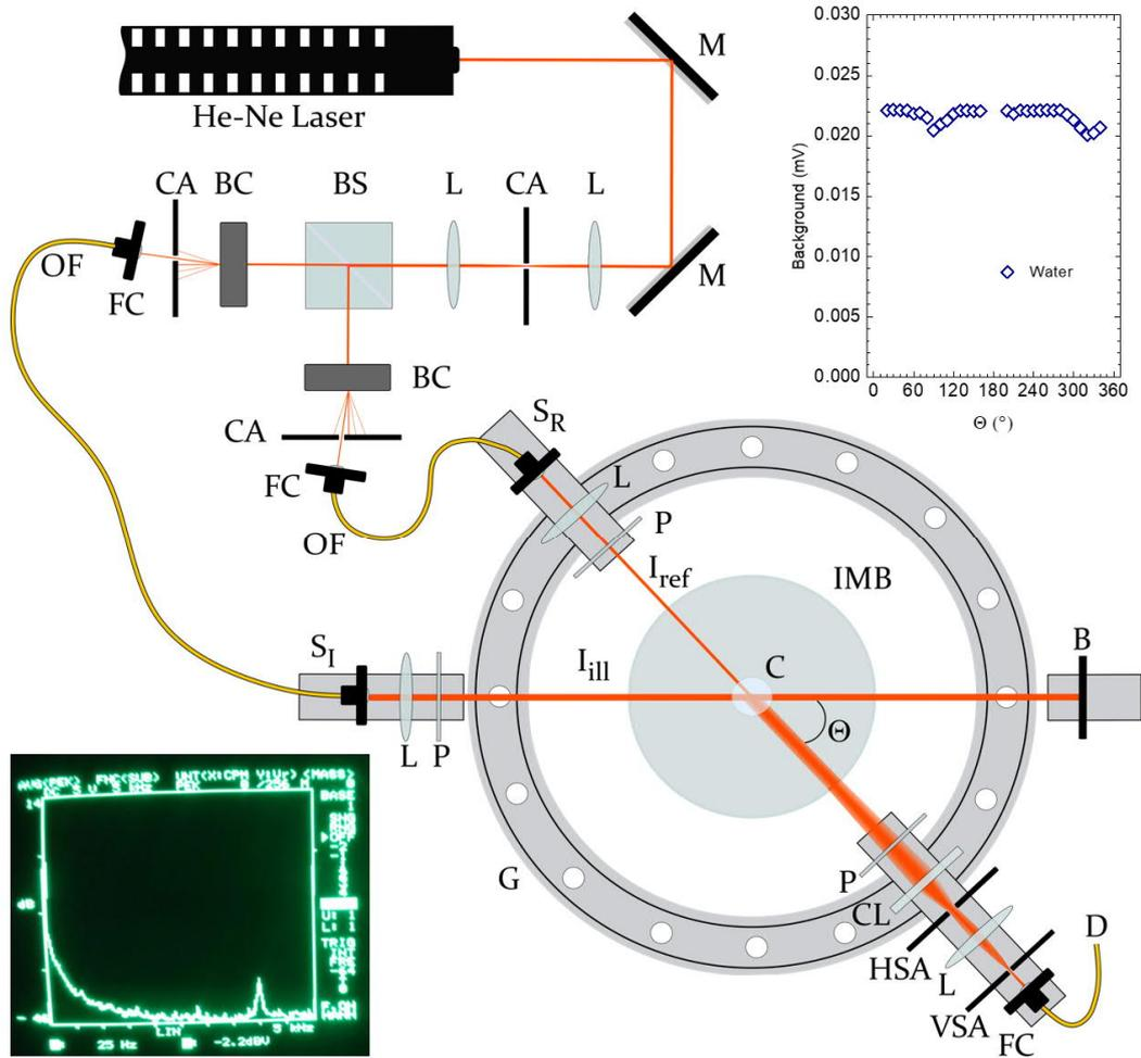
**Fig. 1** Top view sketch of the double arm goniometer with optical and mechanical components. (for details see text). Top right inset: Background intensity reading obtained from an experiment on pure water. Bottom left inset: historical smartphone shot of the first-light signal at the FFT-analyzer showing homodyne and heterodyne signal components.
