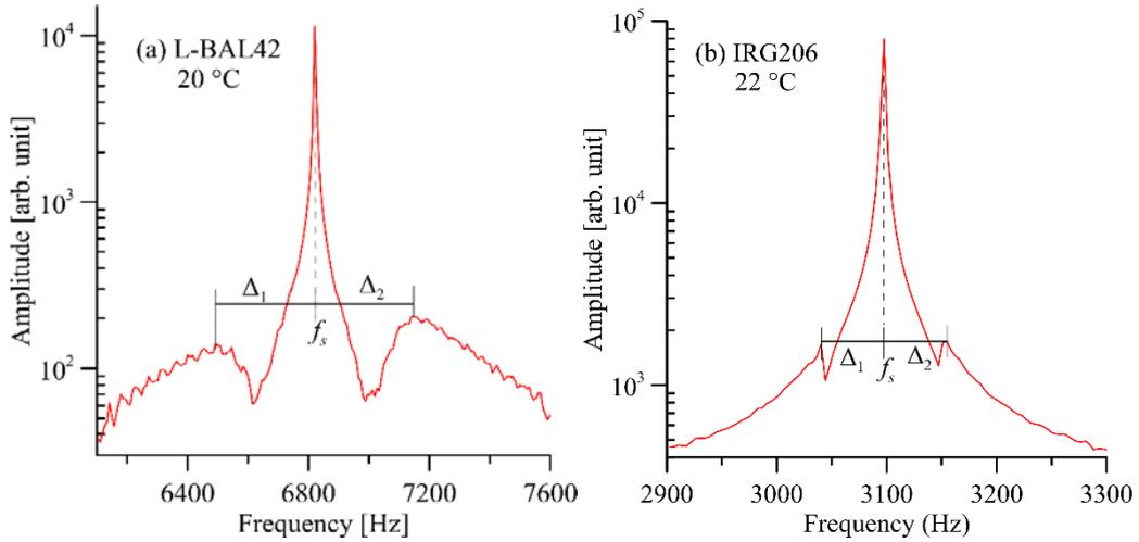
Fig. A2 The Fourier spectrum of the specimen at room temperature. In the plot (a)  $f_s = 6820.68\text{Hz}$  and  $\Delta_1 = \Delta_2 = 320.44\text{Hz}$ ; the Fourier frequency resolutions is 7.63Hz. (b)  $f_s = 3097.50\text{Hz}$  and  $\Delta_1 = \Delta_2 = 57.22\text{Hz}$ ; the frequency resolutions is 3.815Hz
