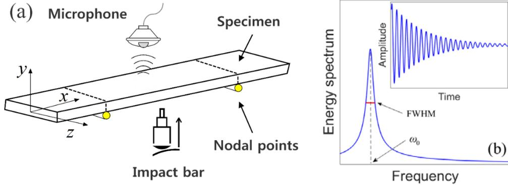
Fig. 3 Sketch of the impulse excitation technique (a) the setup and (b) typical signal and the Fourier transform
