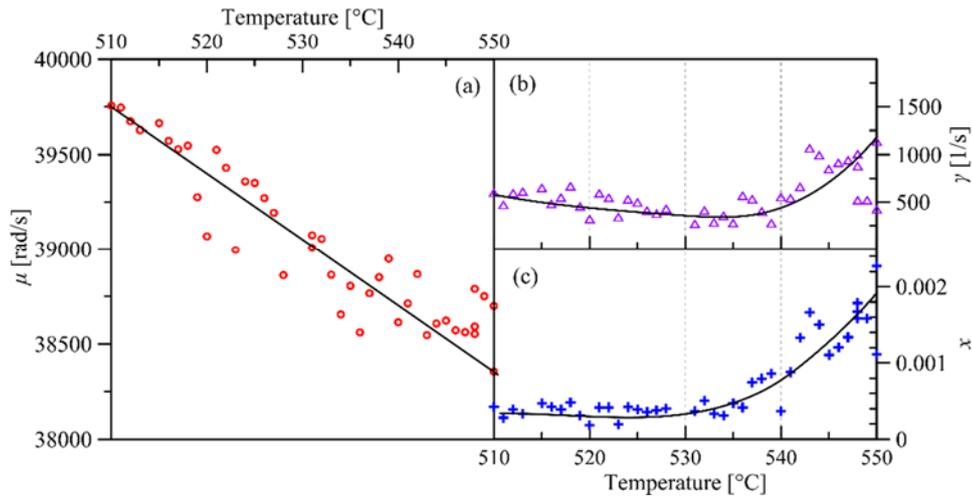
Fig. 6 The temperature dependence of central frequency  $\mu$ , the HWHM  $\gamma$ , and proportion  $x$ . The points are from the theoretical calculation based on experimental data, and the curves are artificial trendlines.
