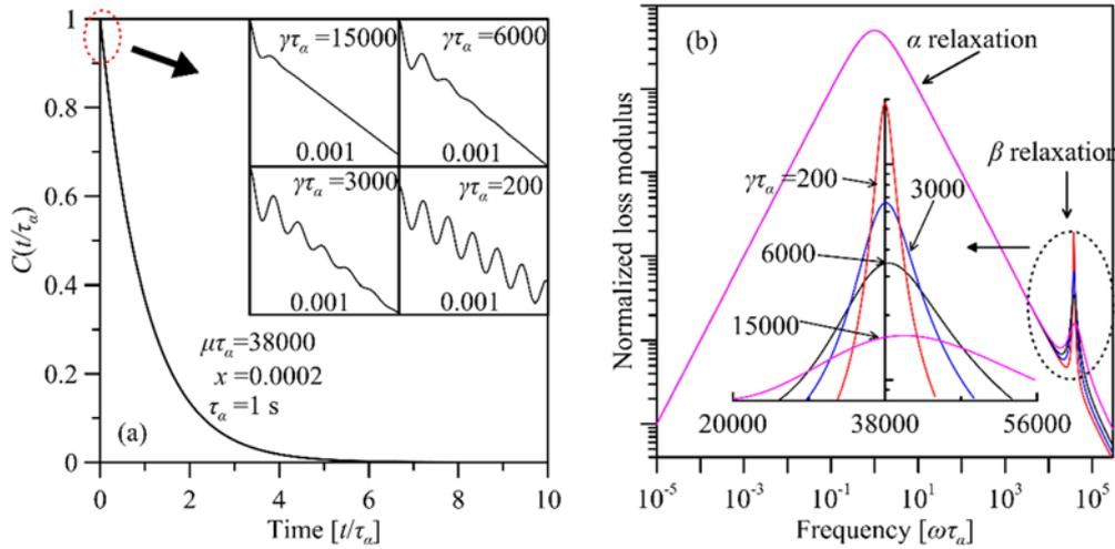
Fig. 1 Examples of stress relaxation (a) and loss spectrum (b) calculated from NMA with Cauchy distribution of  $G(\omega)$ .
