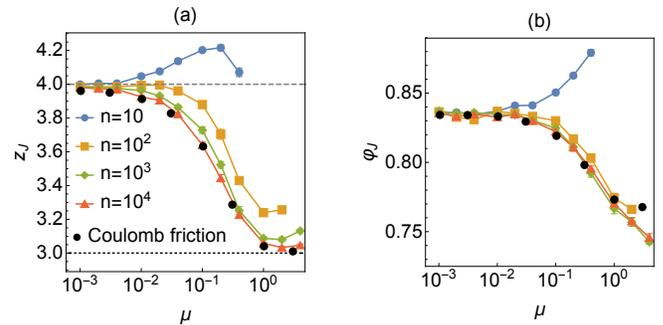
FIG. 3.  $\mu$  dependence for fixed  $\varepsilon = 0.1$  of (a) the contact number per particle at the jamming transition point  $z_J$  and (b) the jamming transition point  $\varphi_J$ . The data for the Coulomb friction model were taken from Ref. [41].
