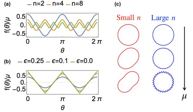
FIG. 2. (a)  $f(\theta)/\mu$  for  $\varepsilon = 0.1$  and several  $n$ . The number of minima increases with  $n$ . (b)  $f(\theta)$  for  $n = 2$  and several  $\varepsilon$ . The triangle wave is recovered when  $\varepsilon = 0$ . (c) Schematic pictures of a particle shape. The shape deviates from the reference disk with  $\mu$ , and the surface becomes rougher for larger  $n$ .
