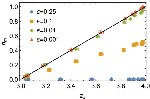
FIG. 6. Relation between  $n_m$  and  $z_J$  for  $n = 10^4$ . Markers denote numerical results. The solid line denotes the theoretical prediction  $n_m = z - 3$  corresponding to generalized isostaticity.
