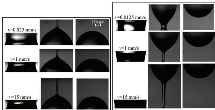
Figure 4: Transfer of water+PAA 1000 ppm from AL to PEMA (left) and from PS to PEMA (right). In each row, the sequence of images shows the initial liquid bridge shape, the shape in the last image before the full receding of the contact line, and the final state. The scale bar applies to all the images. The liquid volume is  $\sim 1.6 \mu\text{l}$ .
