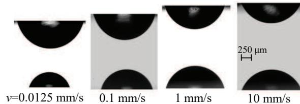
Figure 1: Transfer of glycerol between (AL) (donor surface) and PEMA (acceptor surface) for different stretching velocities. The scale bar applies to all the images. The droplet volume was  $1.2 \mu\text{l}$ .
