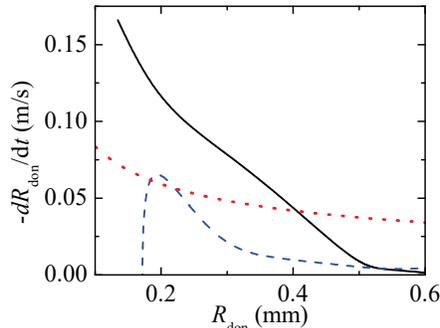
Figure 7: Velocity of the contact line on the donor surface,  $-dR_{\text{don}}/dt$ , as a function of the radius  $R_{\text{don}}$  for water (dashed line) and water+PAA 50 ppm (solid line). The dotted line is one tenth the inertio-capillary speed  $V_{\text{ic}} = (\rho R_{\text{don}}/\gamma)^{-1/2}$ . The donor and acceptor surfaces were PS and PEMA, respectively. The acceptor surface velocity was 10 and 1 mm/s for water and water+PAA 50 ppm, respectively.
