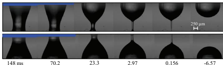
Figure 3: Transfer of water+PAA 1000 ppm from PS to PEMA (top row) and PEMA to PS (bottom row) for  $v = 1$  mm/s. The labels indicate the times to detachment (contact line fully receded). The scale bar applies to all the images. The initial distance between the surfaces was slightly different in the two experiments due to intrinsic contact angle differences between PS and PEMA. The liquid volume is  $\sim 1.6 \mu\text{l}$ .
