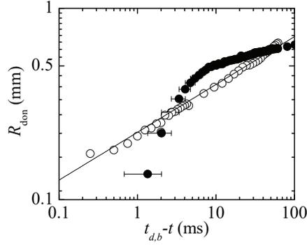
Figure 6: Radius of the contact line on the donor surface,  $R_{\text{don}}$ , as a function of the time to detachment/breakup  $t_{d,b} - t$  for water (open symbols), and water+PAA  $50$  ppm (solid symbols). The solid line corresponds to the fit  $R_{\text{don}} = 0.225(t_{d,b} - t)^{1/4}$  to the water data. The donor and acceptor surfaces were PS and PEMA, respectively. The acceptor surface velocity was  $10$  and  $1$  mm/s for water and water+PAA  $50$  ppm, respectively.
