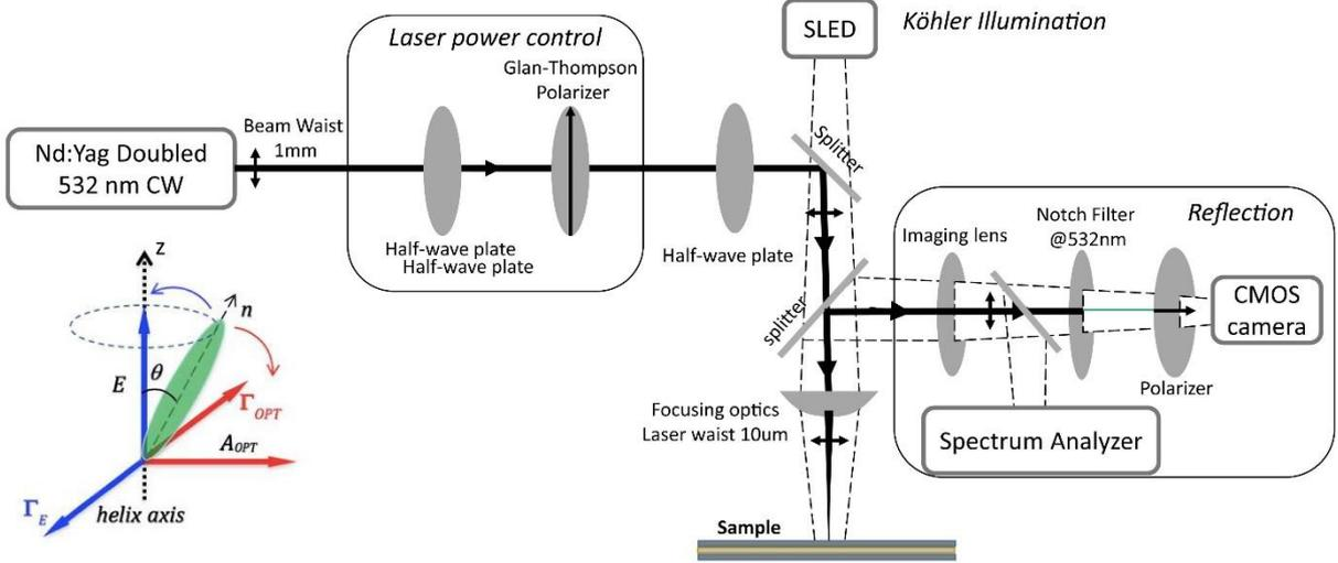
Fig.1 Experimental apparatus. Inset: sketch of the static ( $\mathbf{E}$ ) and optical ( $\mathbf{A}_{opt}$ ) fields and of the corresponding torques.
