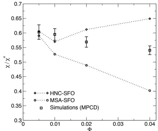
**FIG. 8:** Electrical conductivity  $\chi$  of a 1 – 16 electrolyte, divided by the value at infinite dilution  $\chi^\circ$ , as a function of the volume fraction in nanoparticle  $\Phi$ . Open squares: MPCD simulations ; Open circles and diamonds: Self-consistent Fuoss-Onsager transport theory, with the HNC closure (diamonds), and with the MSA (circles), with the same parameters as MPCD.
