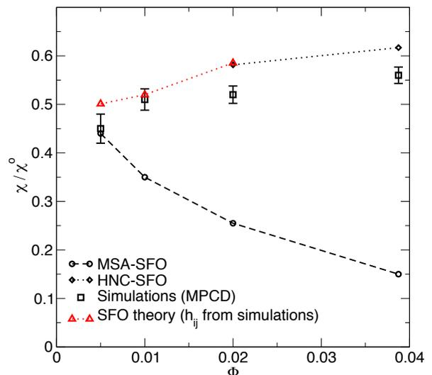
**FIG. 5:** Electrical conductivity  $\chi$  of a 1 – 8 electrolyte, divided by the value at infinite dilution  $\chi^\circ$ , as a function of the volume fraction in nanoparticles  $\Phi$ . The nanoparticles have a diameter of 1.05 nm. Open squares: MPCD simulations ; Fuoss-Onsager transport theory, with total equilibrium pair correlation function  $h_{ij}^\circ(\mathbf{r})$  computed with MPCD simulations (triangles), HNC (diamonds), and MSA (circles).
