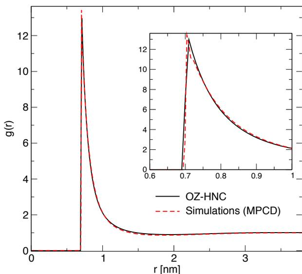
**FIG. 4:** Pair radial distribution function  $g(r)$  between the nanoparticles and the counterions, in the case where the nanoparticle is highly charged ( $Z_{NP} = 8$  for a diameter  $\sigma_{NP} = 1.05$  nm), for a volume fraction in nanoparticles equal to 0.02. The black curve corresponds to the results of integral equations (HNC), while the red dashed line corresponds to the results of the simulations (MPCD).
