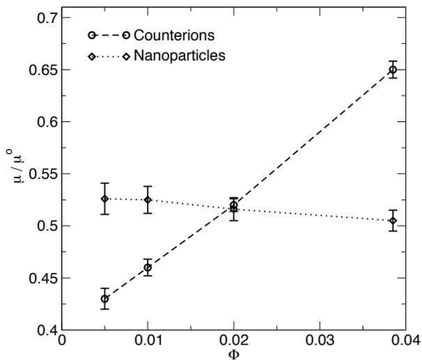
**FIG. 6:** Electrophoretic mobilities  $\mu$  of charged particles of a 1 – 8 electrolyte, divided by the value at infinite dilution  $\mu^\circ$ , as a function of the volume fraction in nanoparticle  $\Phi$ . The nanoparticles have a diameter of 1.05 nm. The values have been computed from MPCD simulations.
