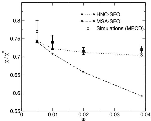
**FIG. 2:** Electrical conductivity  $\chi$  of a 1–4 electrolyte, divided by the value at infinite dilution  $\chi^\circ$ , as a function of the volume fraction in nanoparticle  $\phi$ . Open squares: MPCD simulations; Open diamonds and circles: Self-consistent Fuoss-Onsager transport theory, with HNC closure (diamonds), and MSA closure (circles).
