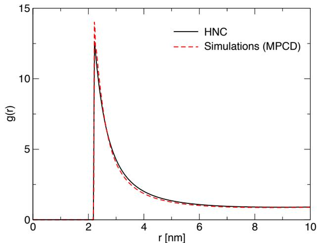
**FIG. 7:** Pair radial distribution function  $g(r)$  between the nanoparticles and the counterions, in the case where the electrolyte is highly asymmetric ( $Z_{NP} = 16$  for a diameter  $\sigma_{NP} = 4.1$  nm), for a volume fraction in nanoparticles  $\Phi = 0.01$ . The black curve corresponds to the results of integral equations (HNC closure), while the red dashed line corresponds to the results of numerical simulations (MPCD).
