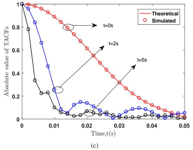
Fig. 3. Theoretical, simulated, and measured TACFs under (a) opposite direction I, (b) opposite direction II and (c) right turn at different time instants.
