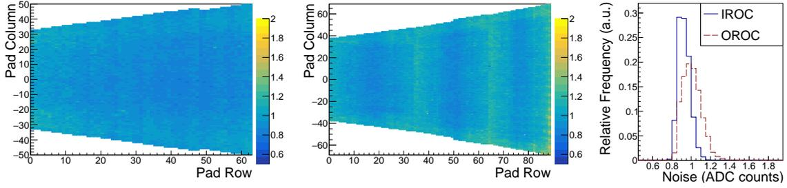
Fig. 1. Noise performance of TPC readout chambers on one TPC sector. From left to right: IROC noise map, OROC noise map, IROC noise distribution (blue, solid line) and OROC noise distribution (red, dashed line).
