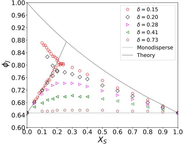
FIG. 1. Jamming density,  $\phi_J$ , as a function of the volume concentration of small particles,  $X_S$ , for different values of the size ratio,  $\delta$ . The extreme  $X_S$  values (0 and 1) correspond to monodisperse systems where  $\phi_J = \phi_{RCP} \approx 0.64$  indicated by the dashed horizontal line. Solid lines represents the analytical result of Eq. (1) [21].
