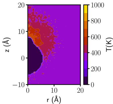
FIG. 3. Distribution of water temperature produced by the periodic inversion of the  $C_{60}$ -X dipole direction ( $\tau = 0.5$  ps). Cylindrical coordinates are employed, with a radial distance  $r$  to the axis defined by the center of the  $C_{60}$  molecule and the X atom, and a height  $z$  with origin at the center of the  $C_{60}$  molecule, with the X atom located at  $r = 0$  and  $z = 5.96$  Å.
