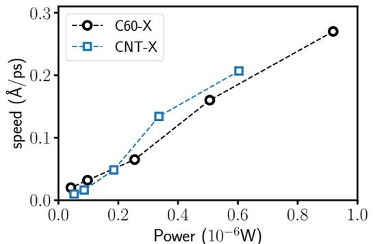
FIG. 2. Speed of  $C_{60}$ -X and CNT-X molecules as a function of the power absorbed. The values for  $C_{60}$ -X result from a multiple regression of the MSD dependence using Eq. 1 [27]. In contrast, the speed of CNT-X is calculated from the net displacement of the molecule before it reaches the edge of the confining nanotube.
