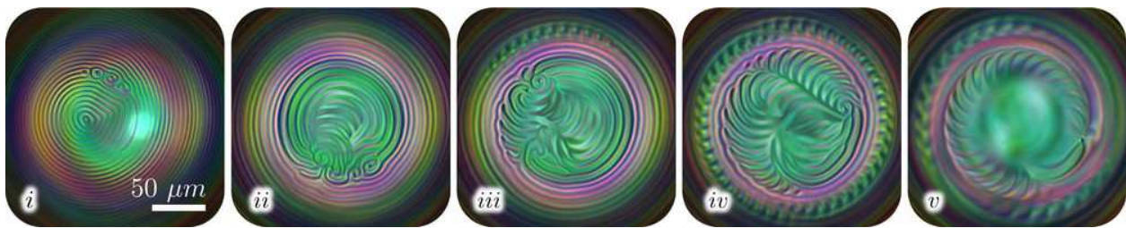
FIG. 4. A homeotropic CLC shell left to equilibrate for one month has two focal conic domains at its poles, with additional defects in the thinnest region of the shell (i). During the homeotropic to planar anchoring transition, the focal conic domains unwind and widen to create greater planar anchoring at the shell surface. As the transition continues, stripes begin to locally undulate with a 2P_0 periodicity (iii-iv), where P_0 = 5 \mu\text{m} . At the end of the transition the planar state is reached, with remnant undulations on the shell. Reproduced from Tran et. al. , Supplemental Video 6 [8].
