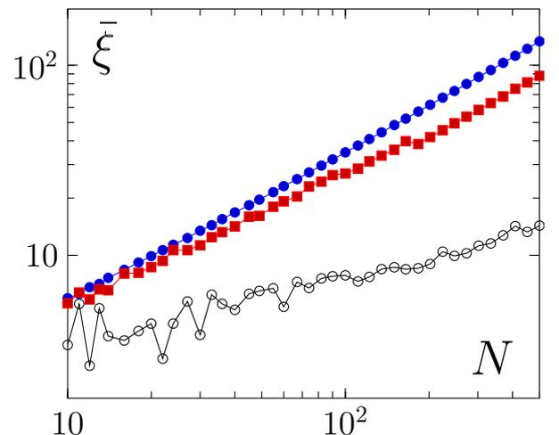
FIG. 4. Average inverse participation ratio  $\bar{\xi}$  as a function of number of ions for the Cirac-Zoller case  $K = 0$  (blue dots), KAM case  $K = 0.0154 \approx K_c/3$  (red squares) and the Aubry phase  $K = 0.1386 \approx 3K_c$  (black circles). The algebraic fit  $\bar{\xi} = aN^b$  for  $\omega_{tr} = 0.014$  gives respectively the value of exponent:  $b = 0.796 \pm 0.0029$  (Cirac-Zoller case),  $b = 0.696 \pm 0.0049$  (KAM case),  $b = 0.349 \pm 0.021$  (Aubry case).
