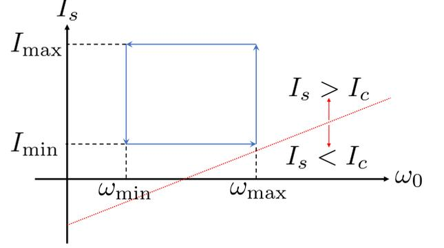
FIG. 2: Illustration of the rectangular loop in  $(\omega_0, I_s)$ -space that gives rise to the geometric phase. The dotted red line separates the subcritical ( $I_s < I_c$ ) and supercritical ( $I_s > I_c$ ) regions.
