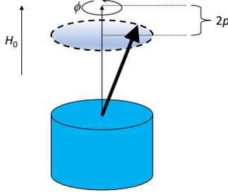
FIG. 1: Illustration of the set-up that is considered: a uni-axial single-domain magnet into which spin current (not shown) is injected. The external field with magnitude  $H_0$  points in the  $z$ -direction. The magnetization dynamics is parametrized in terms of the azimuthal angle  $\phi$  and the power  $p$ . The power determines the projection of the magnetization direction onto the  $z$ -axis.
