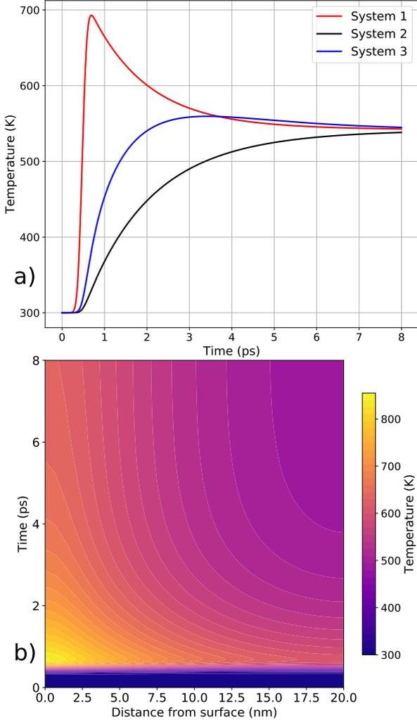
Figure 2: Example of a 3-temperature simulation and the output of two visualization methods: a) `v.average()` and b) `v.contour('1')` described in the text. Here a 20 nm ferromagnetic nickel thin film, heated by a femtosecond laser source is under consideration. The physical parameters are taken from Ref. [2].
