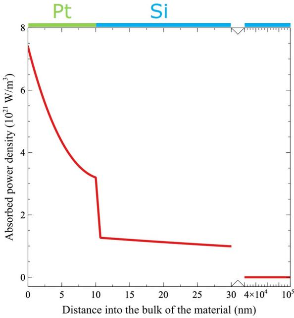
Figure 4: Local power absorption for the platinum/silicon system under consideration, calculated via the transfer matrix method implemented in NTMpy. Here a p-polarized laser pulse with a wavelength of 400 nm, hitting the sample at a 45° angle with a fluence of 6 mJ/cm<sup>2</sup> and a FWHM of 0.1 ps is considered.
