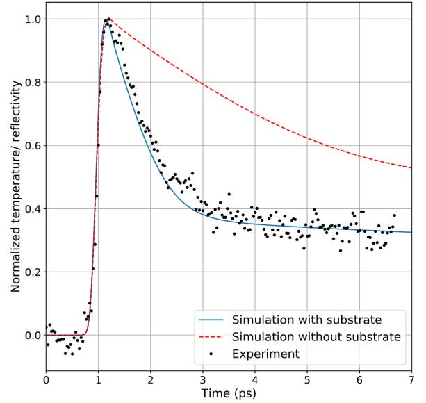
Figure 5: Experimental data of a reflectivity measurement (symbols) compared to the simulated temperature dynamics of a platinum thin film on a silicon substrate (solid line) and free-standing (dashed line). A linear relation between the change in temperature and change in reflectivity is assumed, and they are normalized to the maximum change. The simulation parameters for the materials are taken from Table 1.
