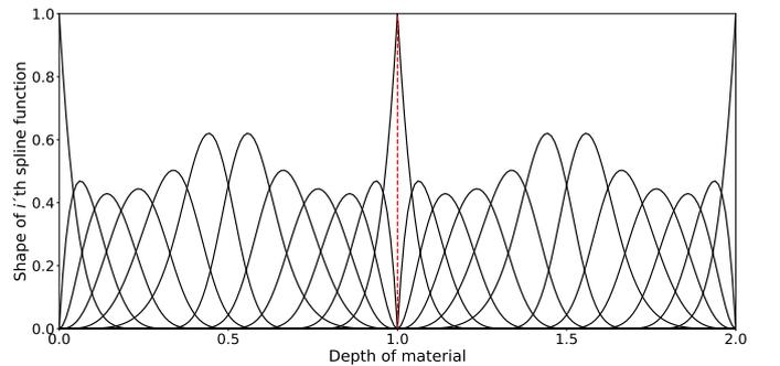
Figure 1: A set of order 5-continuous B-Splines for a two layer system, used to represent the solution in space, where each layer has a length of 1.
