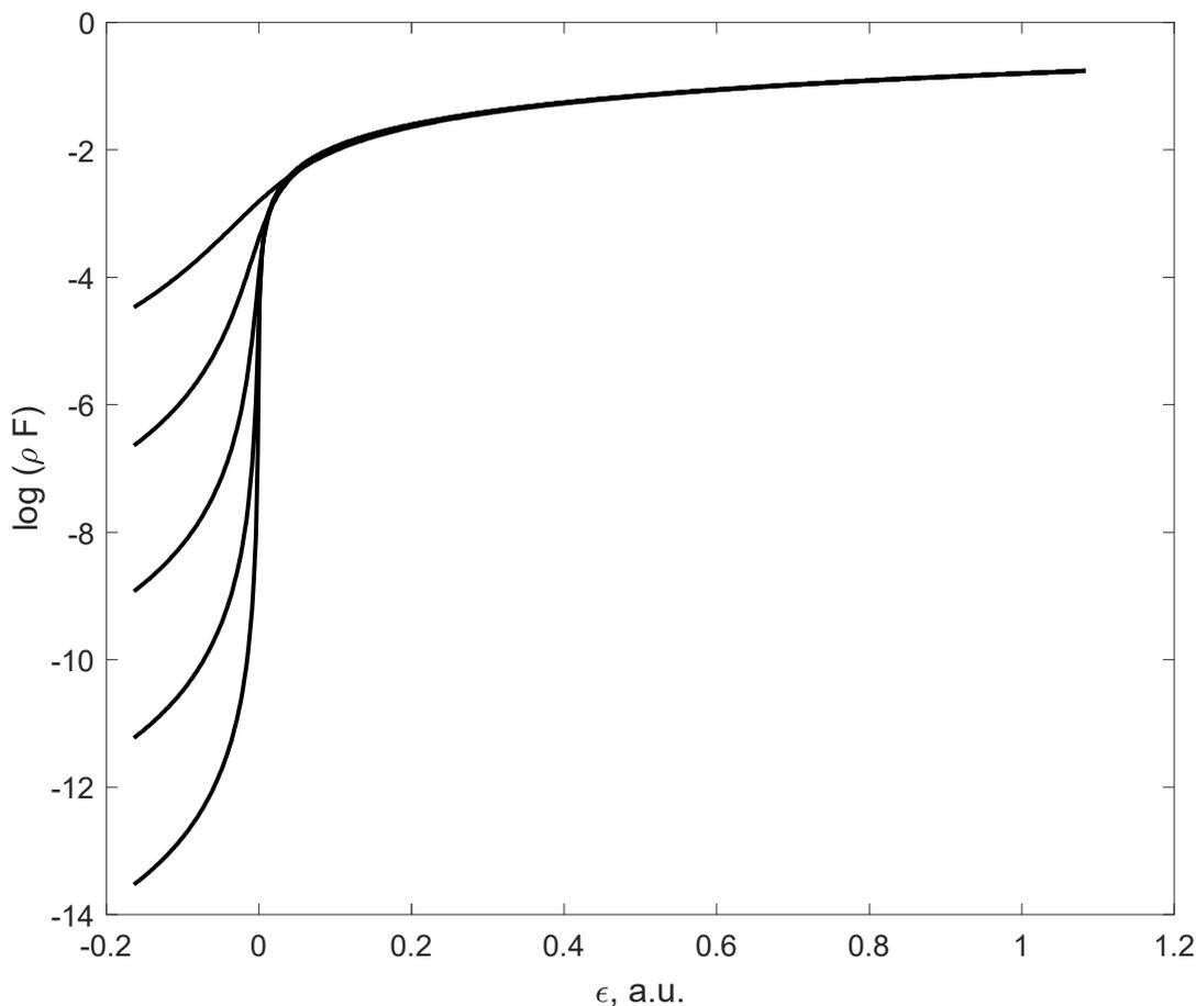
**Fig. 2.** The density of states multiplied by the value of the blocking field for fields with the strength  $F = 10^{-2}, 10^{-3}, 10^{-4}, 10^{-5}, 10^{-6}$  a.u. depending on the energy. The curves are arranged from top to bottom in descending order of field strength.
